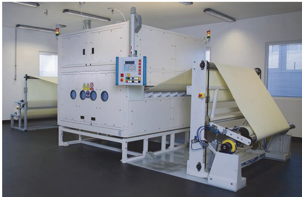
Fig. 10. Nozzle-less production electrospinning line (Nanospider™).
