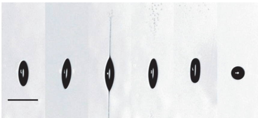
Fig. 1. The droplet (radius, 24 micron) is imaged on a vertical charge-coupled-device array to determine and control its vertical position in the levitator, and on a photomultiplier that detects instability-onset, quadrupole-shaped oscillations of the droplet. These oscillations trigger a signal to a flashlamp that fires after a predefined delay, \Delta t [1].
